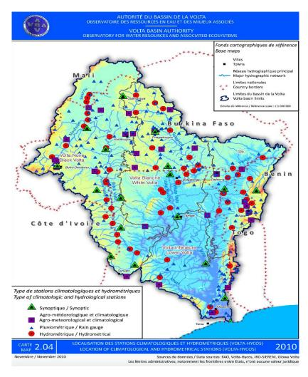
Figure 3: Hydro stations of the Volta Basin<sup>28</sup>
